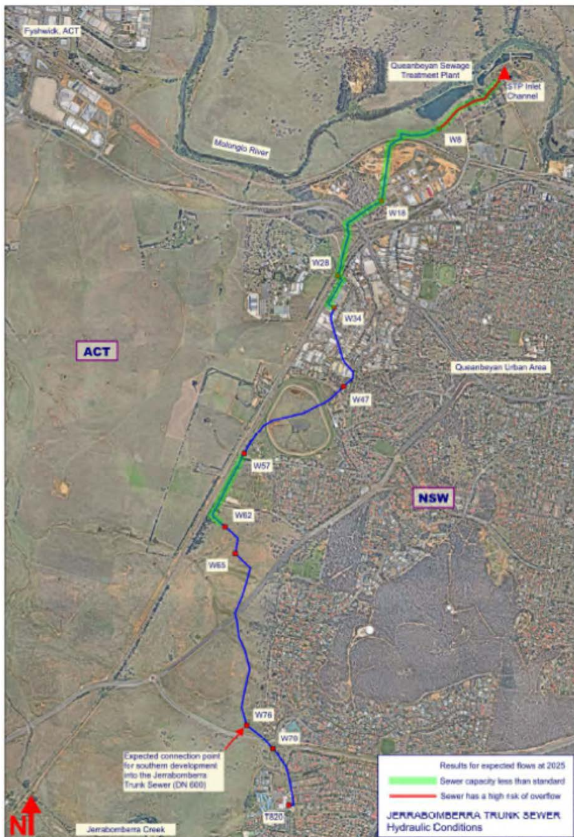
Figure 5-2 Expected condition of the Jerrabomberra trunk sewer after 10 years (Image from South Jerrabomberra Structure Plan 2013)
