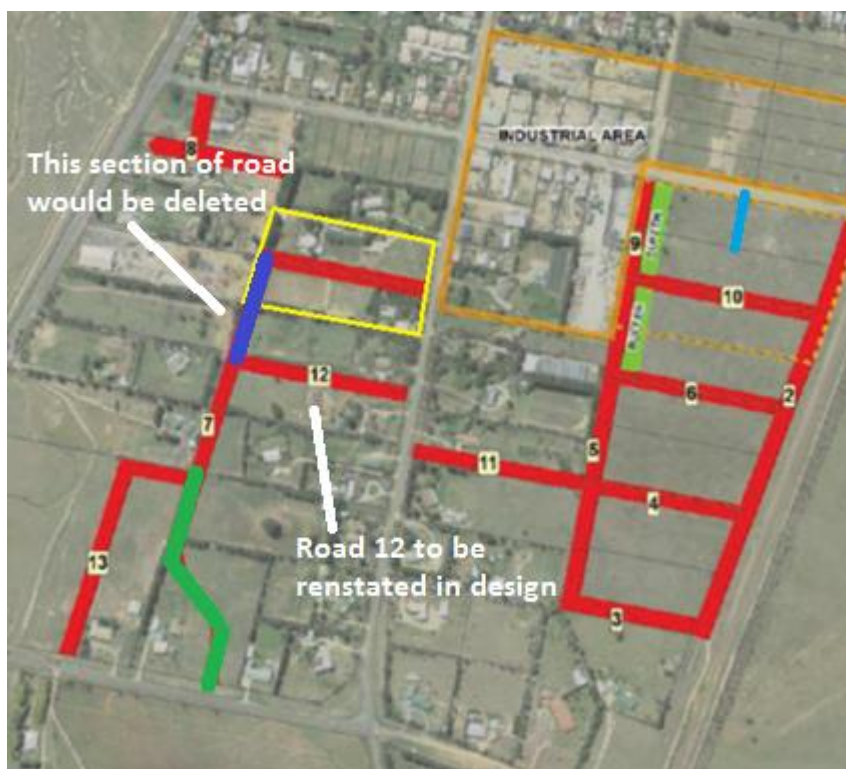
Figure 4 – Option 2 showing extent of southward road extension which would no longer be required if cul-de-sac was implemented and reinstatement of Road 12.
