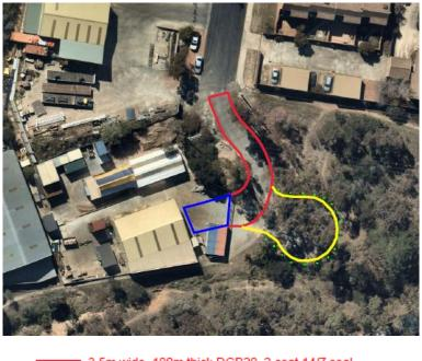
3.5m wide, 100m thick DGB20, 2 coat 14/7 seal.
