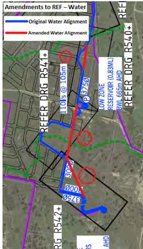
Figure 2 – Existing water main shown in blue – Proposed amendments shown in red.
