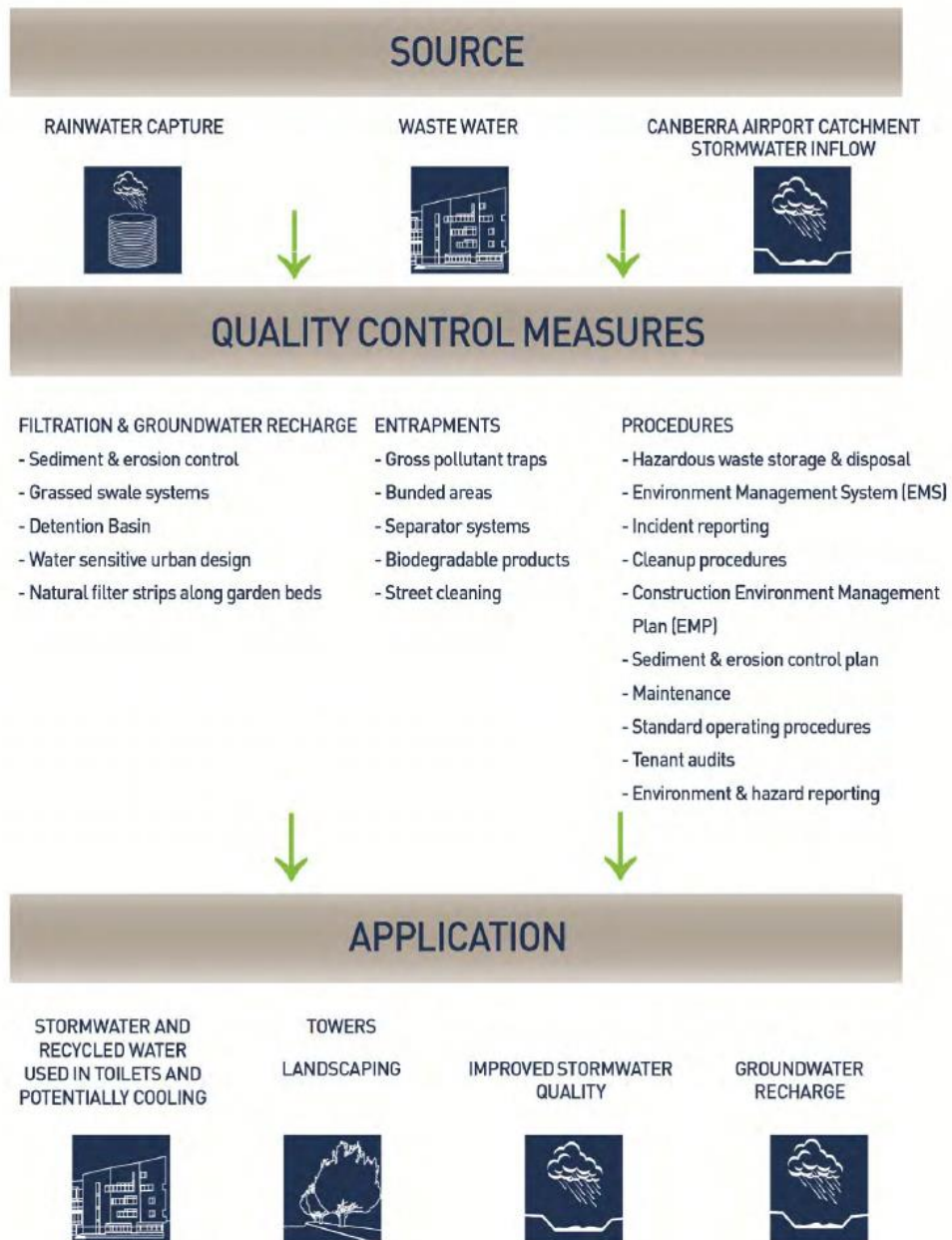
Figure 3.1 - Non-potable water flowchart
