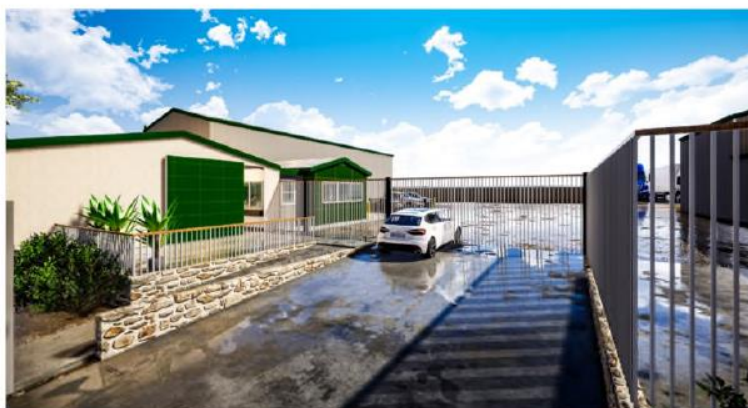
Figure 8: This proposed view shows the new entry off Duncan Street. A new concrete driveway will be installed to replace the existing 2 entry points. This will allow easier truck and vehicle access. This will also increase pedestrian safety and visibility. A new access ramp is provided providing an AS1428.1 compliant entry point to the site, Elements of new landscaping coupled with elements of local stone cladding will also offer an enhancement to the streetscape and overall built quality Simple new metal fencing will also secure the site.
