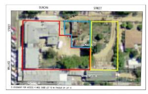
Initial subdivision plan proposed in the CMP with proposed Lot 11 including the two corrugated iron sheds. The boundary between proposed Lot 12 and proposed lots 11 and 10 should be 900mm east of the wall of the corrugated iron shed.
