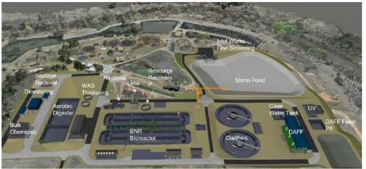
Figure 9: Overview of the Queanbeyan STP Upgrade (existing plant in background)
