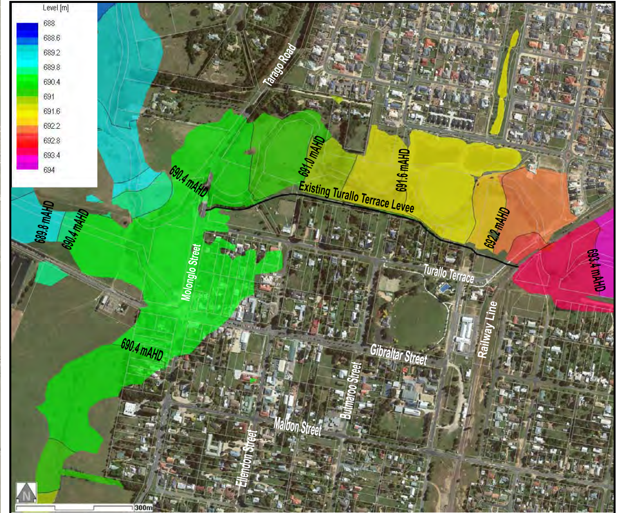
INSET Close-up of flooding in the vicinity of the Village NOTE The variation in peak 5 year ARI flood levels are shown at a reduced contour interval of 0.3 metres ( the larger view is shown at 1 metre intervals ).
