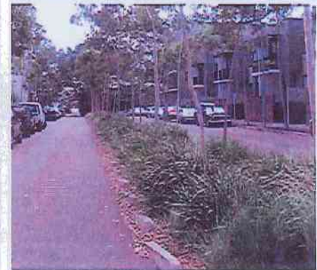
Indicative street median bioretention treatment
