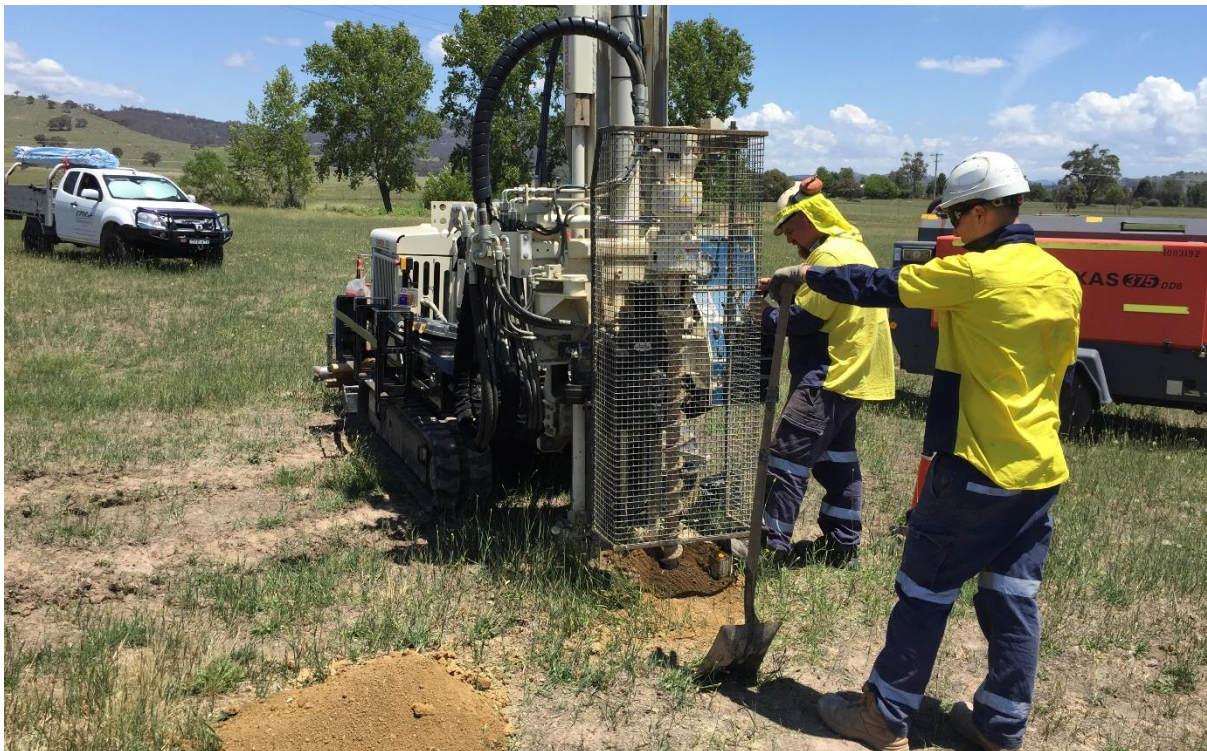
Figure 4 – Drilling borehole MW02B. Boreholes were excavated using a solid stem flight auger attachment from 0.5m bgl until auger refusal in bedrock, below which, deeper boreholes (MW02B and MW09B) were drilled into bedrock using an air hammer methods.
