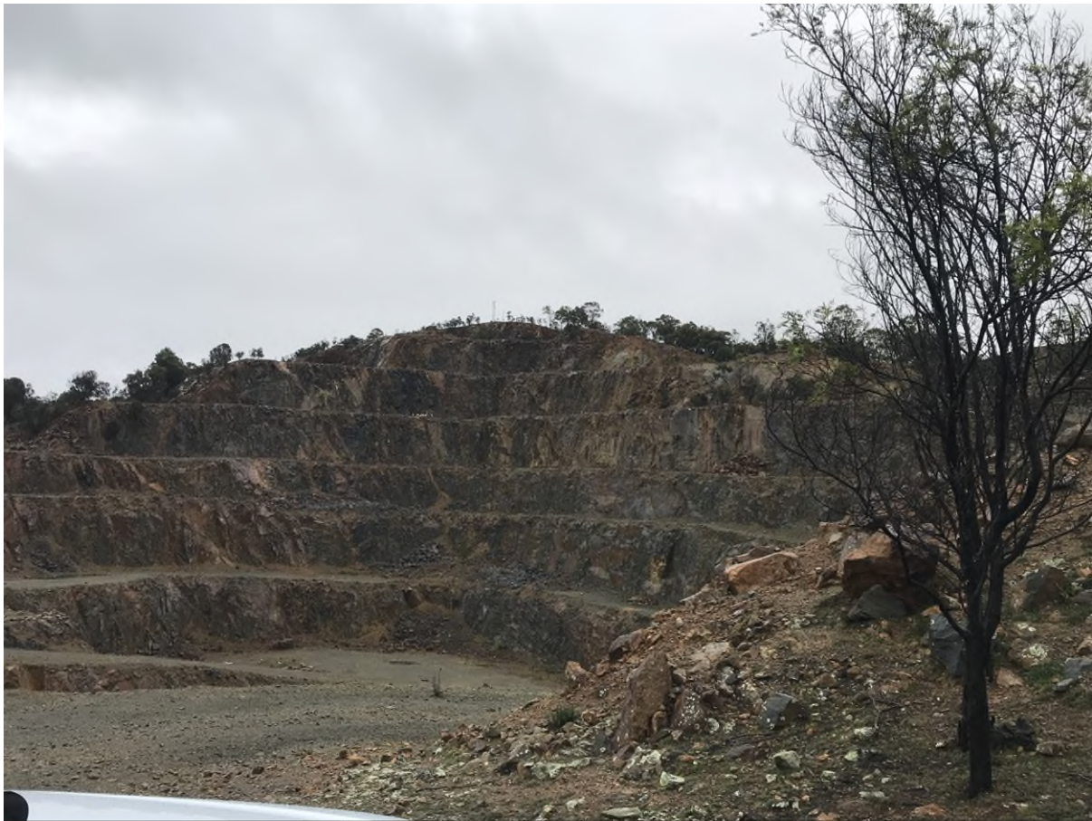
Figure 3: Photo of quarry showing extent of the cut. Benches 10-15m in height.
