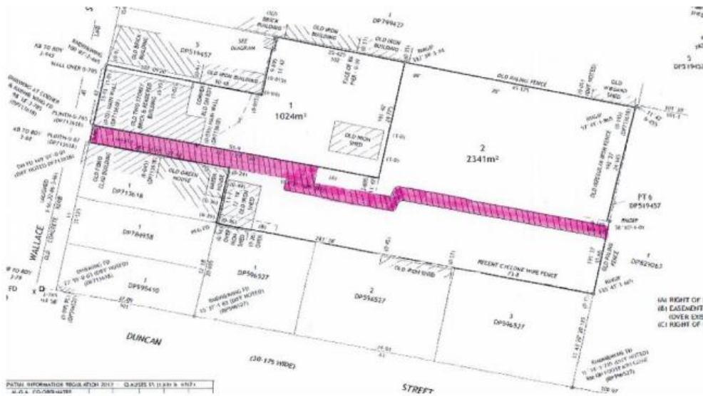
Figure 1 – Right of Carriageway
