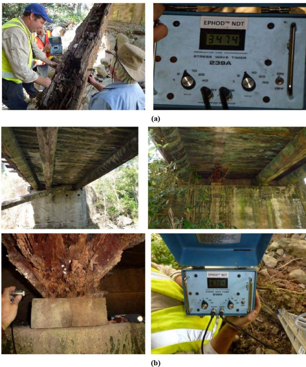
Figure 12-1: Photos showing global failure of a timber log girders. Both failures were caused by advanced decay in the ends of the girders and transverse shear failures. The primary cause of this decay was due to vertical fasteners. These failures were found in elements with SWT values in the 3k \mu s (photos a. above) to 6k \mu s range (photos b. below). Typically, similar bending extreme tensile fibre failures in log girders occur in zones of decay where there are over 2k \mu s SWT values. Similarly, if vast portions of the log girder have SWT values over 3k \mu s the failures may occur.
