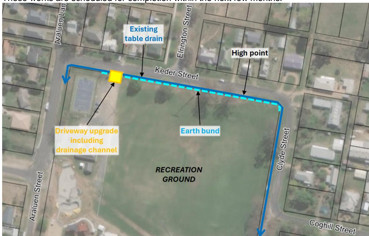
Figure 3: Sketch of Keder Street works
