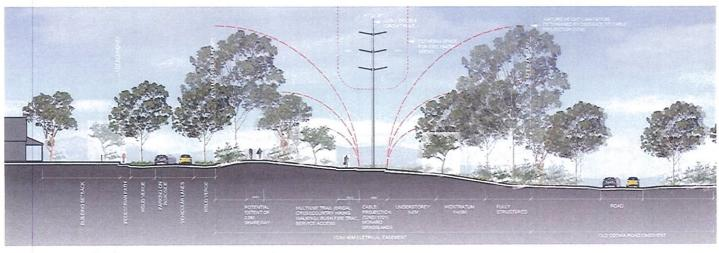
Figure 11: Typical Old Cooma Road Easement Section - Looking South
