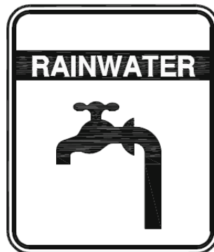
Figure 5: Example rainwater fixture signage (at washing machine and rainwater tank outlets)
